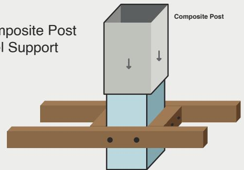
**Installing with Composite Decking**
