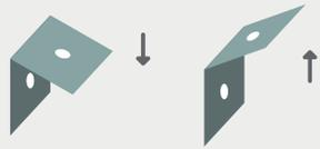
The L-Shaped Brackets can be eased to the required angle by applying pressure
