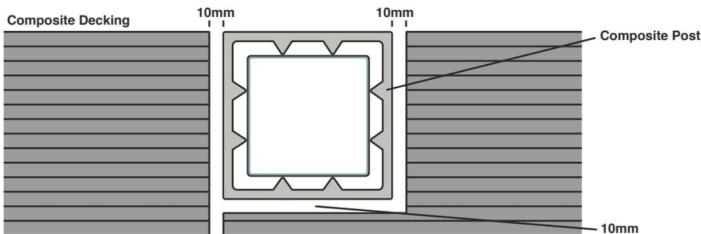
Leave 10mm gaps around Composite Posts to allow for expansion. The gap will be covered by the Post Foot Cover.
