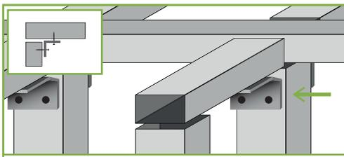
To create steps, cut profiles to required lengths, and connect to down turn supports (fixed to perimeter joist) using angled (L-Shaped) joist connectors.
