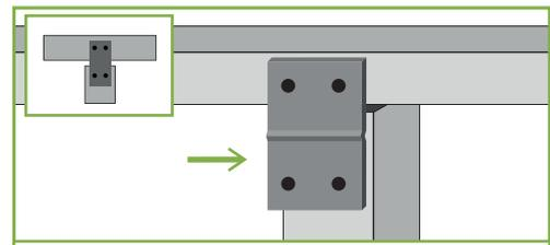
If down turns are required, cut vertical profiles to required length, and connect to perimeter joist using straight joist connectors.
