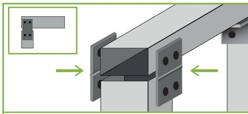
To create down turn for steps, cut profiles to required lengths, and connect using L-Shaped brackets.
